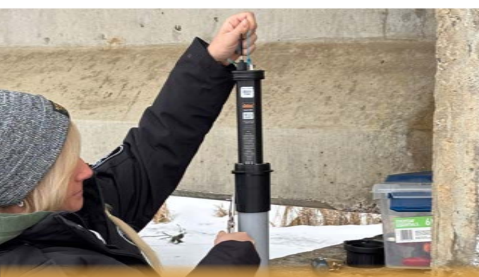
Staff inspecting newly installed water level loggers on the Floodway.
