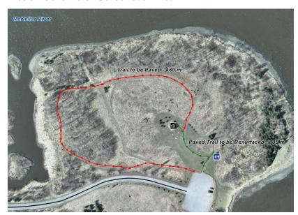
The existing trail network in consideration consists of 480 metres of existing gravel surface that is to be paved. Additionally, there is 105 metres of existing asphaltic surface that is to be regraded and resurfaced. The trail network is expected to meet or exceed the AODA compliance requirements.
