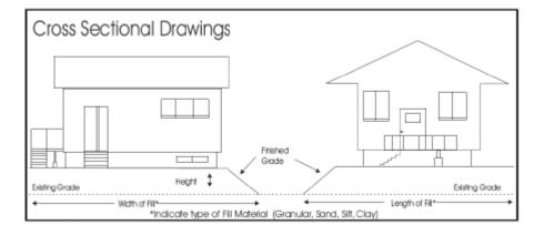
Cross sections must show existing and final grade elevations, existing and finished floor elevations and lowest openings into buildings.
